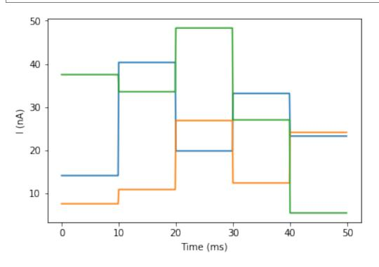
Sure enough, it's different each time. But why? We wrote group.run\_regularly ('I = rand()\*50\*nA', dt=10\*ms) which seems like it should give the same value of I for each neuron. But, like threshold and reset statements, run\_regularly code is interpreted as being run separately for each neuron, and because I is a parameter, it can be different for each neuron. We can fix this by making I into a *shared* variable, meaning it has the same value for each neuron.
