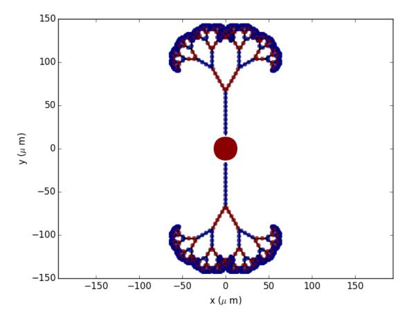
To get more "realistic" morphologies, this function can also be used to create morphologies in 3D where the orientation of each section differs from the orientation of the parent section by a random amount:
