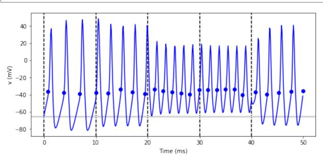
We've replaced the loop that had multiple run calls with a run\_regularly. This makes the specified block of code run every dt=10\*ms. The run\_regularly lets you run code specific to a single NeuronGroup, but sometimes you might need more flexibility. For this, you can use network\_operation which lets you run arbitrary Python code (but won't work with the standalone mode).
