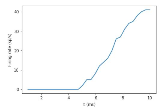
You can see that now there is much less noise and it increases monotonically because the input spikes are the same each time, meaning we're seeing the effect of the time constant, not the random spikes.
