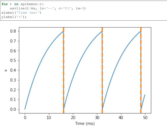
Here we've used the axvline command from matplotlib to draw an orange, dashed vertical line at the time of each spike recorded by the SpikeMonitor.
