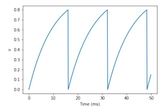
We've added two new keywords to the NeuronGroup declaration: threshold='v>0.8' and reset='v = 0'. What this means is that when v>0.8 we fire a spike, and immediately reset v = 0 after the spike. We can put any expression and series of statements as these strings.
