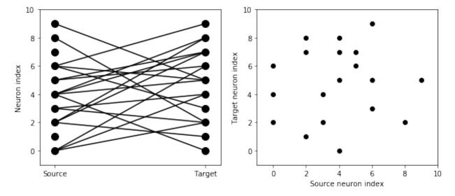
There are two plots here. On the left hand side, you see a vertical line of circles indicating source neurons on the left, and a vertical line indicating target neurons on the right, and a line between two neurons that have a synapse. On the right hand side is another way of visualising the same thing. Here each black dot is a synapse, with x value the source neuron index, and y value the target neuron index.
