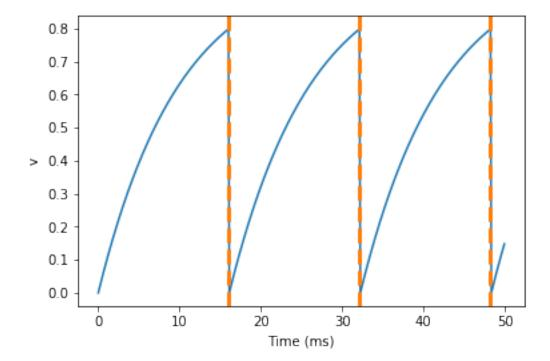
Here we've used the axvline command from matplotlib to draw an orange, dashed vertical line at the time of each spike recorded by the SpikeMonitor.
